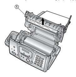
**5** Turn the gear of the blue core (①) in the direction of the arrow until the ink film is tight (②).
